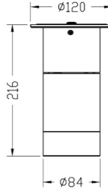
DIMENSION INCLUDES SNOOT OR BEZEL OPTIONS. IF THOSE OPTIONS ARE NOT USED THE SIZE IS REDUCED BY 35mm
